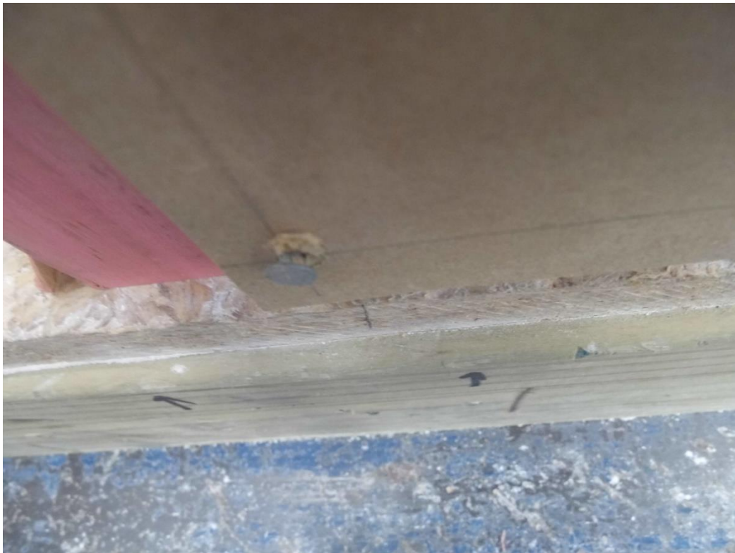
Figure 6. Extraction of the nail fixing at a bottom corner of a 1200 mm long specimen
